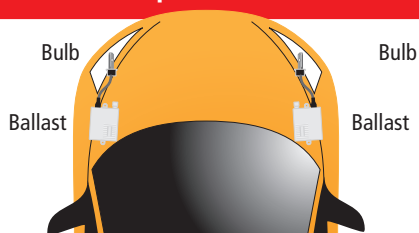
Fig.6 Control unit position
