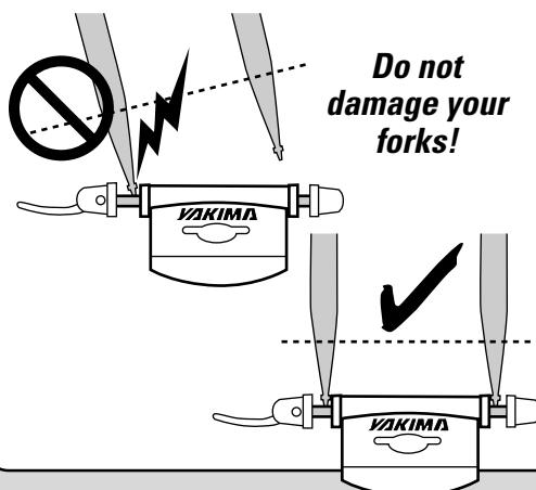
**14** With lever open, tighten nut until the lever closes with firm resistance.
