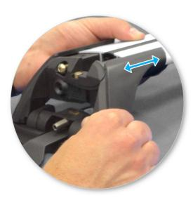
Press adjusting screw to adjust the leg positions on the crossbar.
