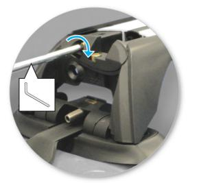
Tighten adjusting screw to 5 Nm (3.7 ft lb) hand tight.
